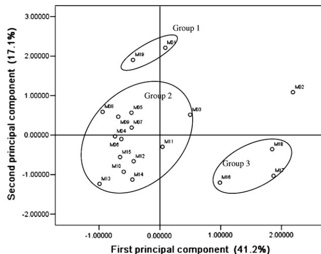
Fig. 3. Scope plot of principal component analysis for relative contributions of the 17 toxic dioxin congeners in the stack gases from MSW incinerators.
