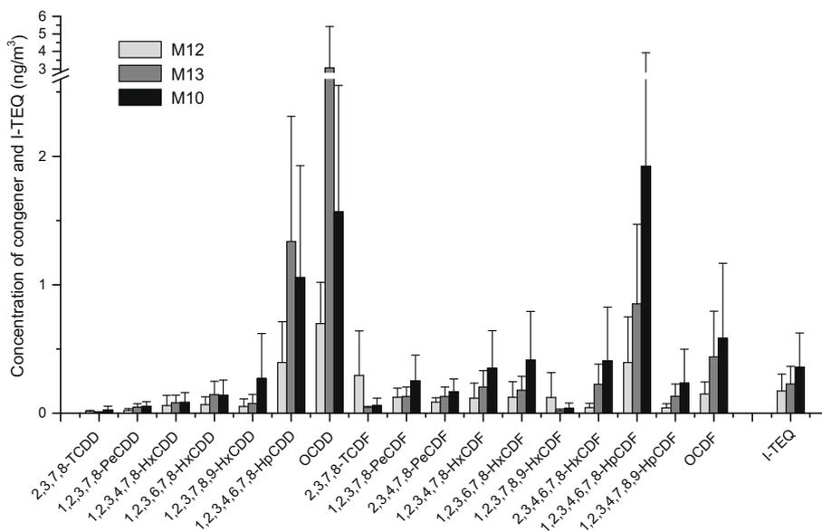
Fig. 2. Emission levels of PCDD/Fs from three home made MSW incinerators built by Weining Co. Ltd.
