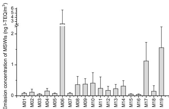
Fig. 1. The emission levels of PCDD/Fs from 19 MSW incinerators in China.
